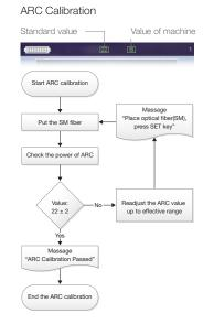
Important: 1) Always use SM fiber only 2) To keep in best splice condition, following the procedure.
